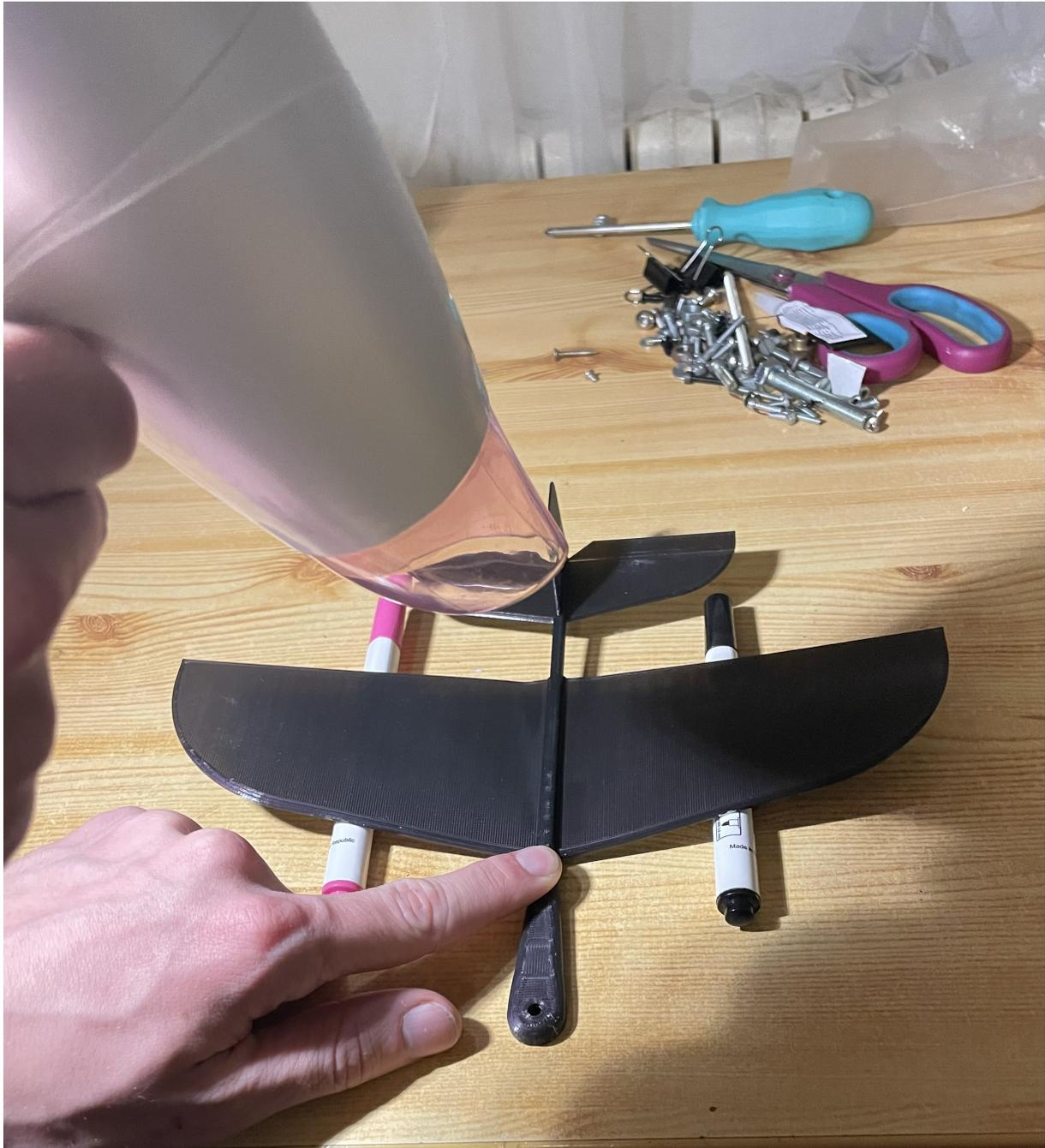
the center of gravity of the aircraft needs to be adjusted for the best result. screw a screw with a diameter of M4 and a length as required into the front hole. according to the photo:
